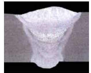
Macro section: Hybrid' technology in V bevel R-H SMAW, F-C FCAW in uphill progression
