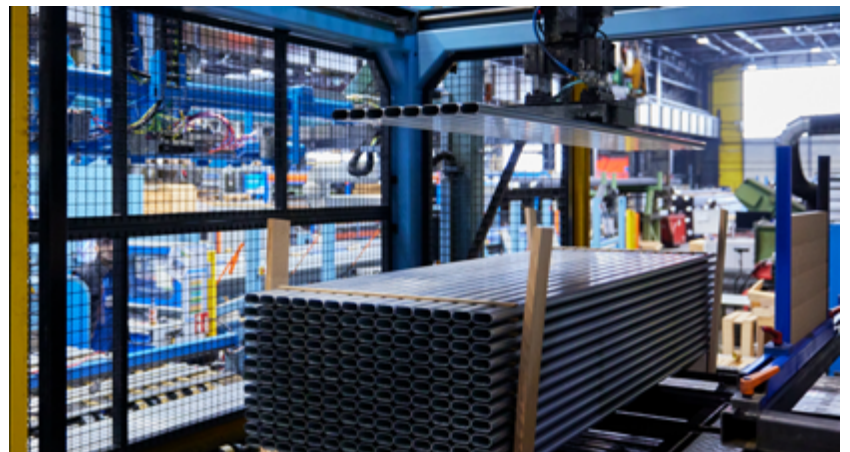
» Automated sorting and bundling
