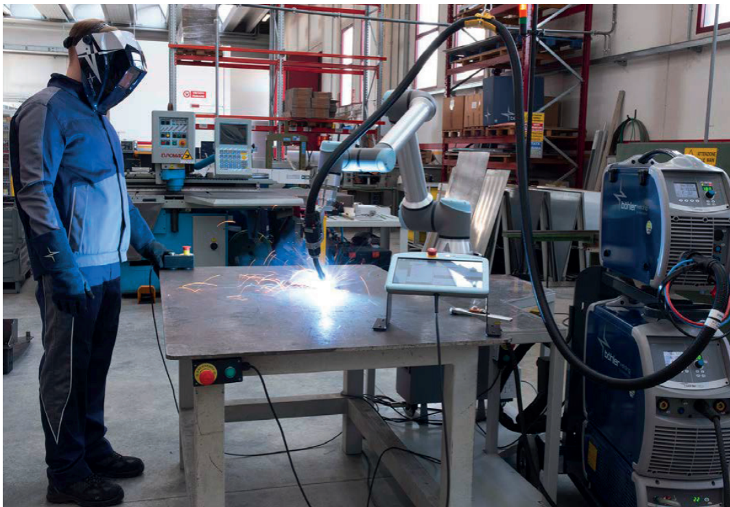
A collaborative robotic welding installation
