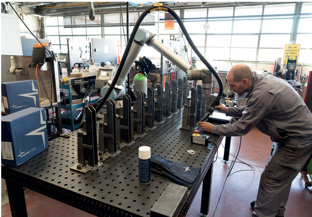
Bracket serial production using CO-BRO® at Bozonet
