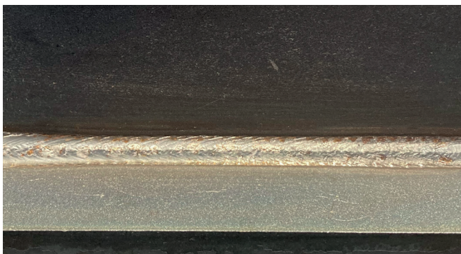
Robotic fillet weld high productivity using non-coppered wire ECOSPARK 420 and process QuickPulse. Pictures show the perfect bead profile without undercuts, good penetration, no spattering and very few residuals such as silica islands on the weld.
