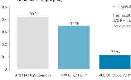
Rail/Wheel Test Rig: Head Check Depth [mm] The excellent characteristics have also been confirmed in the international Heavy Haul Benchmark Test at TTCI. The operational performance of this rail grade is characterized by
