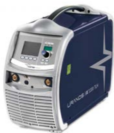
URANOS \propto 3200 TLH / ACDC TIG DC / TIG AC 320 A @ 40% 3x230-400 V 3-320 A 26.0 kg
