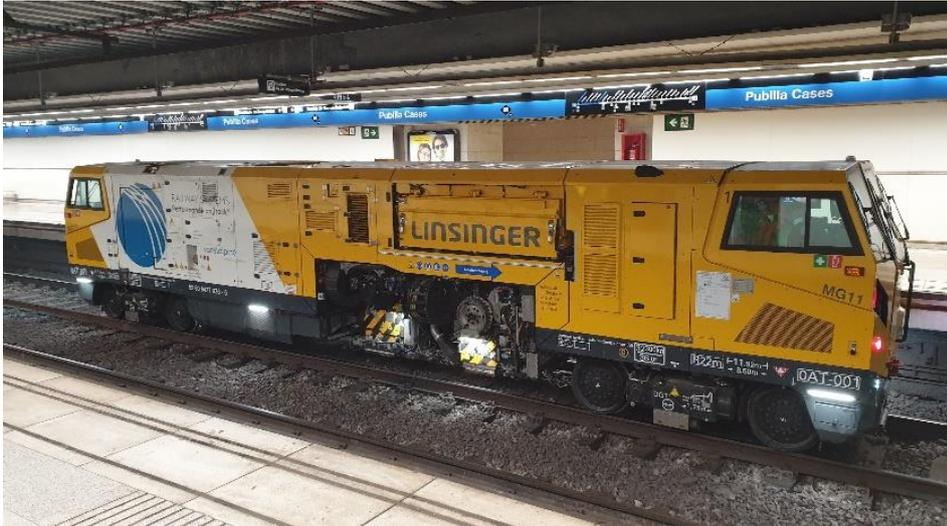
Smart rail monitoring with subsequent rail maintenance by means of milling for the Barcelona Metro were implemented by voestalpine Railway Systems' subsidiary voestalpine Track Solutions Germany and PJM in a holistic service offer.
