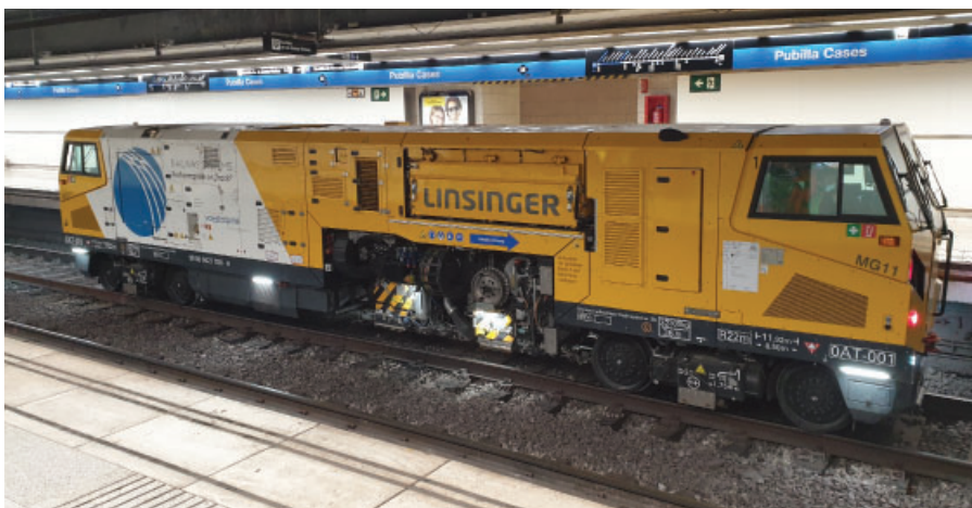
The milling is completed with a MG11 rail milling machine.
