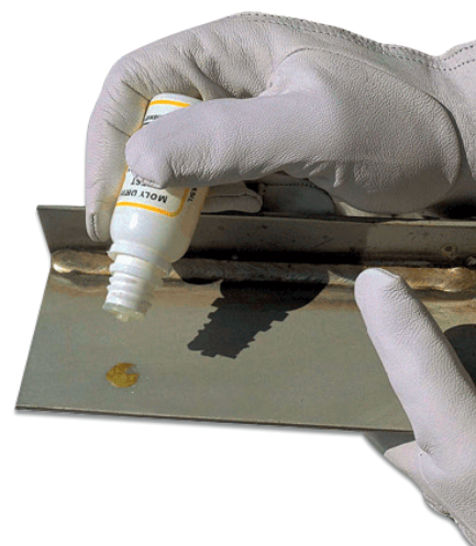
Photo : Showing easy test for differentiating stainless steel grade 304 from 316.
