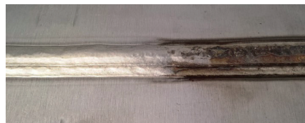
Photo: Usage of Duplex Pickling Spray 250 on LDX 2101 ® welded with Avesta FCW-2D 2205 Considered a difficult combination to pickle.
