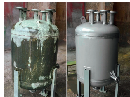
Before After Photos: Pickling of steel grade 321 (1.4541) Temp 5°C with pickling time 90 min.
