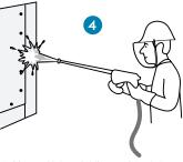
4. Rinse off the pickling residuals by using a high-pressure water jet. Use deionized water for the final rinsing of sensitive surfaces. The waste water should be neutralized before discharge.
