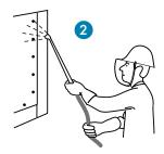
2. Stir the pickling spray before usage. Apply with SP 25 and spray evenly over the entire surface.
