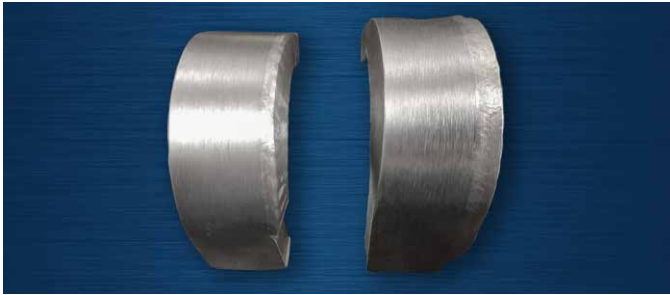
Bend test according to ASME IX and ASTM E190-14:
