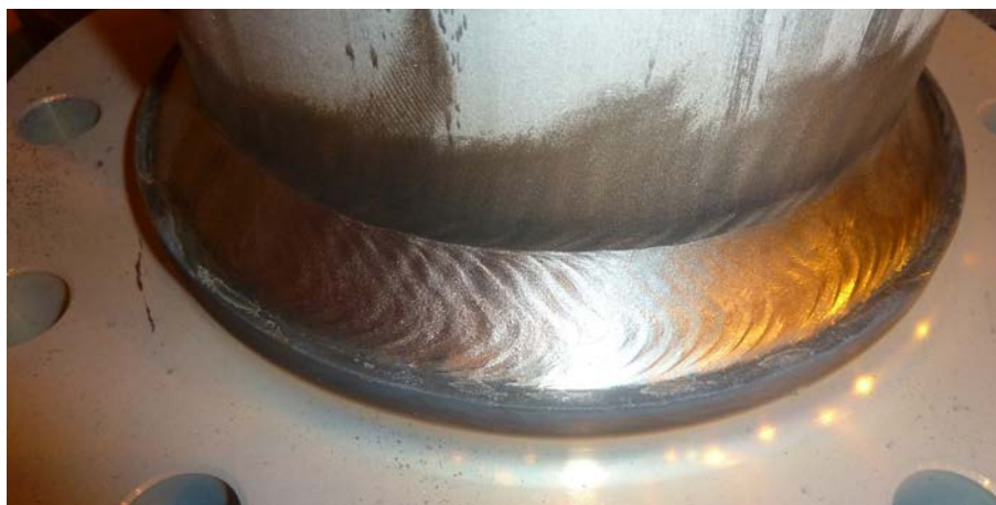
Fillet weld in flat position (PB / 2F). The base material is AISI 304L and the filler FOXcore 308L-T0 DG. Ø 1.2 mm.
