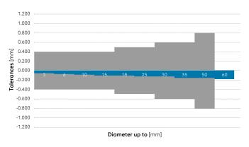
Hot-rolled wires to DIN EN 10017 Cold-drawn wires to DIN EN 10278
