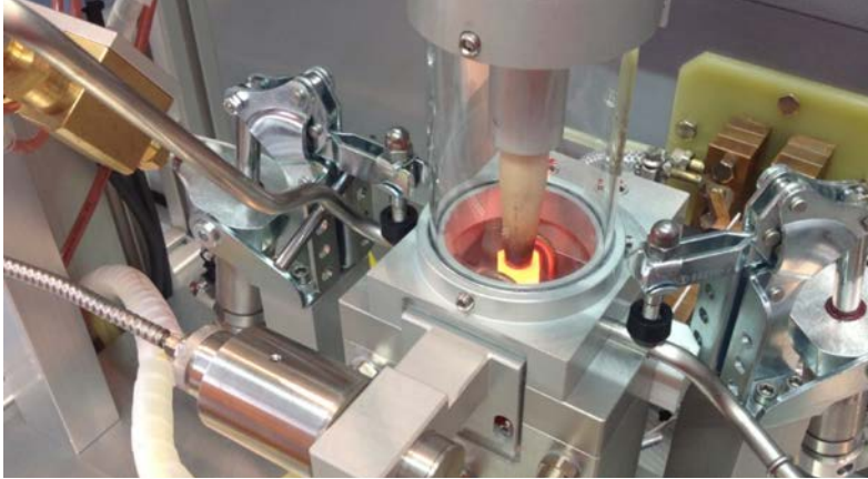
Gas-shielded induction brazing by using Nitrogen; alloyed steel tube construction, Brazing alloy A 200 L (with kind permission of IEW Induktive Erwärmungsanlagen; www.iew.eu )
