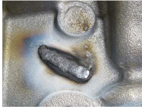
Short stringer bead before slag is removed
