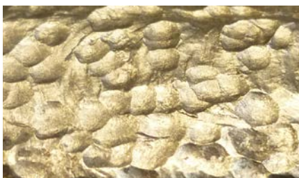
Hammered out weld metal
