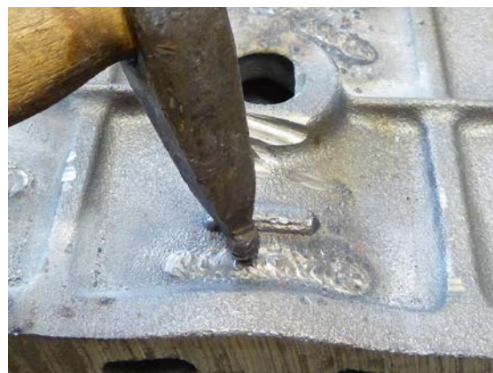
Short stringer bead after slag is removed
