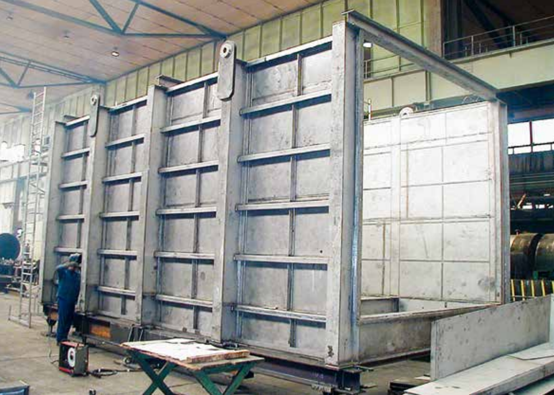
Stainless steel construction ready for pickling.
