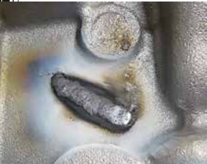
Short stringer bead before slag is removed
