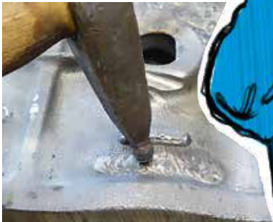
Short stringer bead after slag is removed
