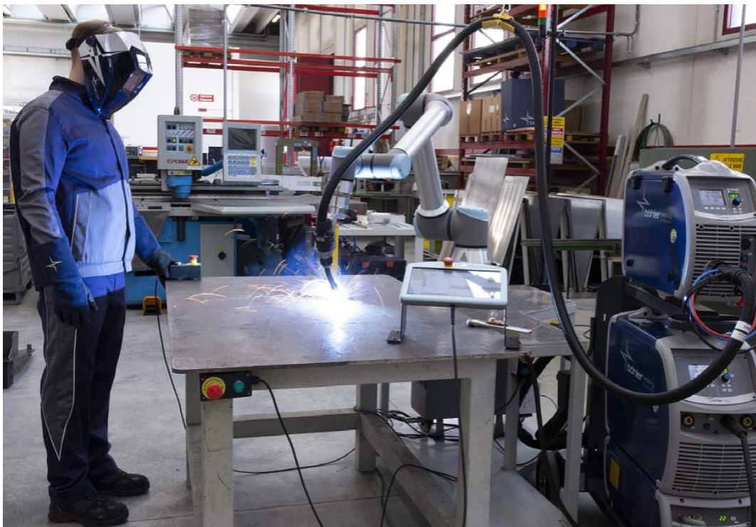
A collaborative robotic welding installation
