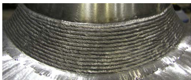
Figure 17: Grade 91 tee-connection manufactured by shielded metal arc welding
